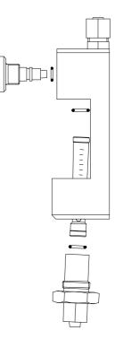
The plastic plugs of the measuring glass are carefully dismounted and the float element is removed. For cleaning isopropyl alcohol is perfectly suited.
