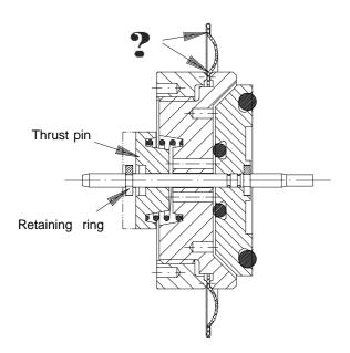
For dismounting the diaphragm, special clamping wrenches (part no. 31617) or face spanner (spigot Æ 3mm und 4mm) are used. The diaphragm must be exchnaged if it is defective or embrittled. The thick O-rings in the diaphragm disc should always be exchanged. In doing so, be careful not to damage the O-ring groove.
