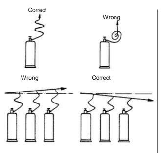
As a result of temperature variations, chlorine gas may condense to liquid chlorine in the overpressure system. Therefore a uniform ambient temperature must be provided. A room heating is recommended.
