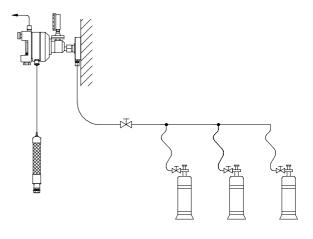
A collective pipe connects all cylinders forming one pressure system so that chlorine is supplied simultaneously from all cylinders. For connecting the chlorine cylinders with the collective pipe flexible copper pipes are used. Each flexible copper pipe is equipped at the end with an cylinder auxiliary valve which is closed when exchanging the cylinders so that the escape of chlorine gas is avoided.
