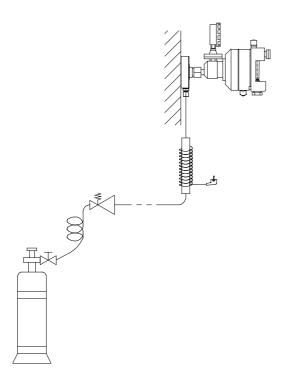
Theoretically the vacuum could amount to a maximum of 1 bar, but the ejector primes only at a technically reasonable slight vacuum. Therefore the pressure loss resulting from pipe friction in the vacuum lines must not be higher than 50 mbar. The following table shows the required line cross section in relation to the length of line and the metering capacity.
