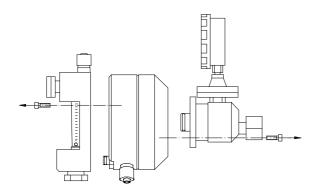
For dismounting the diaphragm disk the thrust pin is pushed down and the retaining ring is removed using a long nose plier.
