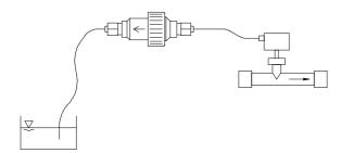
The check is carried out under vacuum contrary to the flow direction. Connect a transparent tubing to the open side and immerse its end into water. The water may not rise in the tubing.
