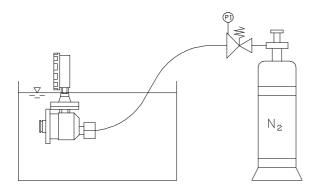
Neither at high pressures (e.g. 6 bar) nor at low pressures (e.g. 0.5 bar) bubbles must rise.
