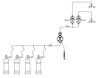
In this example the long distance is carried out in DN12, and for the relatively short unit connections a 8/12 PE tube is used.
