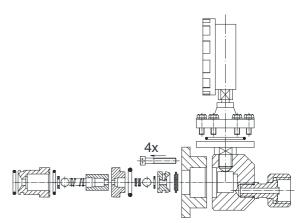
For cleaning purposes the pressure gauge flange can be opened without problems by unscrewing the six screws so that the silver diaphragm becomes visible. It must be wiped off carefully using a soft cloth. Do not use a sharp-edged toll at any rate.
