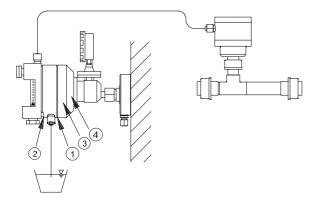
After switching on the ejector, the water level in the tubing rises only a few centimeters and then remains constant. The ball in the flow meter rises, then drops slowly and indicates zero after a short time.
