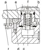
The intake valve is reassembled as follows: All components are slightly lubricated with Vaseline or silicone grease.
