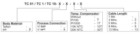
TOSHCON Online Conductivity Probe Model TC-01 / TC-1 / TC-10 are available in Teflon body with SS Electrode & Teflon Insulator for in line or submersible application.
