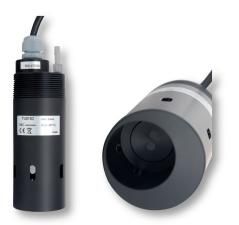
Turbidity probes TU 8182 has been designed for submersible measures, and it is equipped with a built-in nozzle for autocleaning by means of pressured air blasts.
